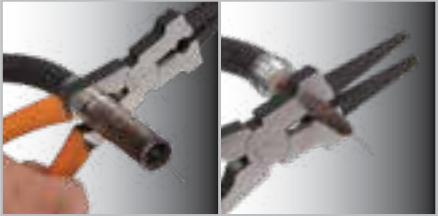
Nozzle removal & installation Tip removal and installation
