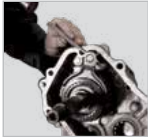
Pin Punches are used for driving out and removing already loosened pins & keys after initial movement by a solid or starting punch
