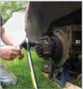
Torque multiplier used for lug nuts
