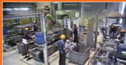
Pressure die casting - PLC controlled semi automatic equipment
