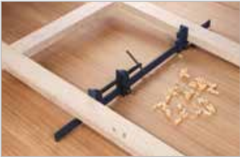
Duo Bar used for internal clamping
