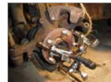
3 Jaw Puller used for removing tyre hub
